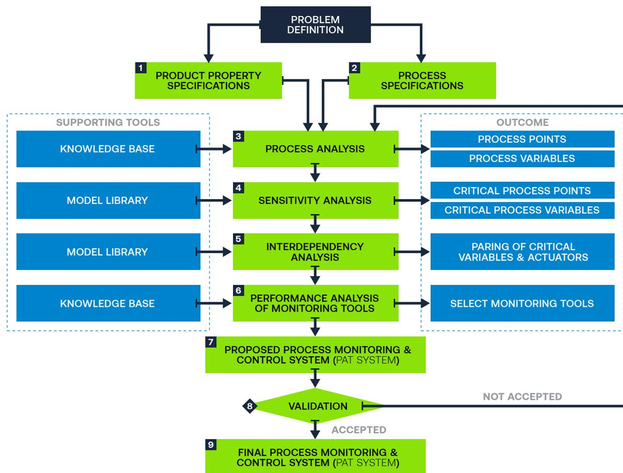
Figure 1: Overview of the nine-step methodology for PAT system design (extracted form [Assessment])
