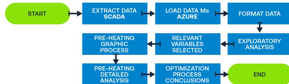
Figure 3: Data capture and pre-processing pipeline for building a digital twin for a pharmaceutical drying process<sup>38</sup>
