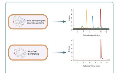
Precise genome editing of the wild producer strain makes it possible to remove the specific parts of biosynthetic gene clusters responsible for producing toxic by-products. With fewer impurities to remove and less of those that do remain, processes complexity and costs associated with purification and disposal simply disappear along with the non-target peaks in the analytical results.
